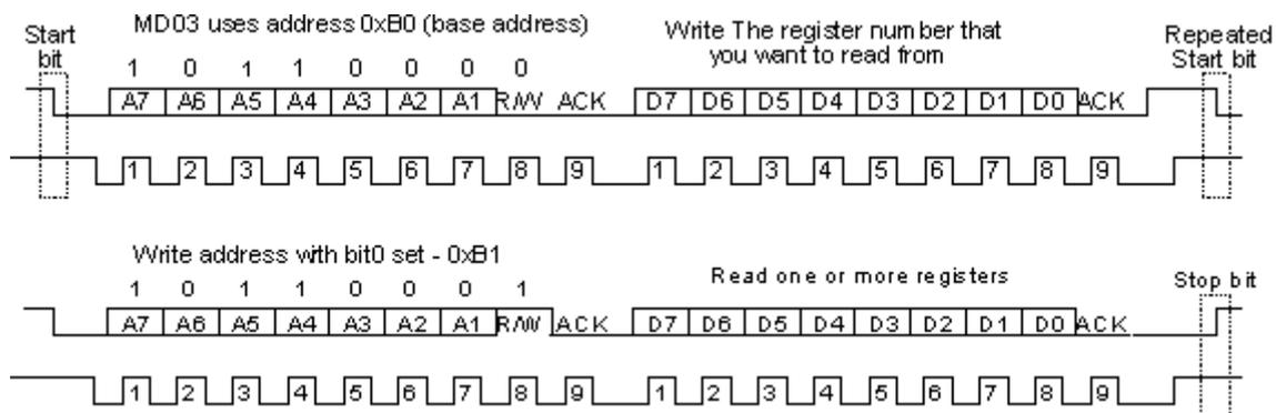
I2C communication protocol with the MD03 module is the same as popular eeprom's such as the 24C04. To read one or more of the MD03 registers, first send a start bit, the module address (0XB0 is the base address) with the read/write bit low, then the register number you wish to read. This is followed by a repeated start and the module address again with the read/write bit high (0XB1). You now read one more registers.
